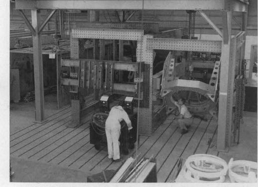
BIG STATIC JIG helps provide fundamental data on stress-strain problems. This roomful of steel girders in Bldg. 860 is used to test assemblies up to 25 feet long, is an important tool in evaluating mechanical properties of units. Adjusting control console, left, is Andy Imrisek, and right, Elmer White, both of 1612-2.
